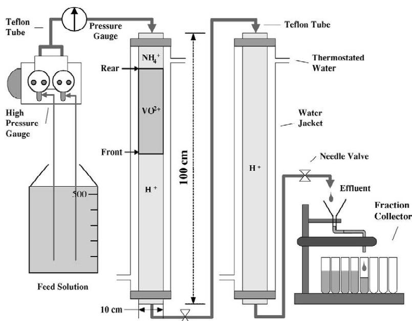
Fig. 1. Schematic separation system by displacement chromatography.
